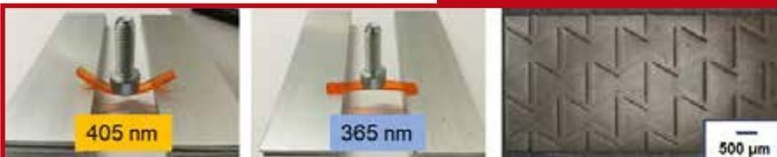
printed at 365 nm (Fig. 1). This allows the printing of multi-material structures, without the need for a change of the resin vat (Fig. 2).
