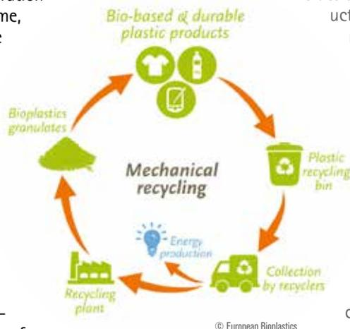
Intelligent recycling processes and loops enable the prolonged sustainable use of materials and significantly contribute to resource efficiency. Besides the re-use of products, the mechanical recycling (i.e. the retrieval of polymeric material from plastic waste) represents a very sustainable recovery option for polymeric materials. Mechanical recycling allows for preserving the polymeric structure and the material value in terms of feedstock and polymerization energy.
