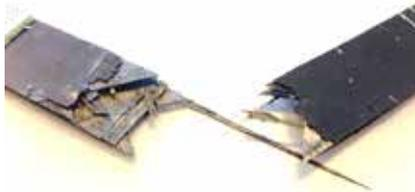
Fatigue failure of a quasi-isotropic laminate
