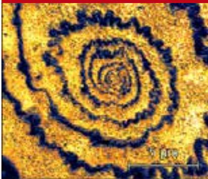
Fig. 2: AFM image of calcium carbonate crystallized on cellulose acetate
