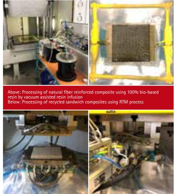
Above: Processing of natural fiber reinforced composite using 100% bio-based resin by vacuum assisted resin infusion
