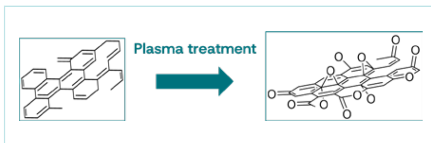
Effect of plasma treatment on surface chemistry of carbon material
