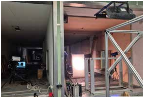
Fig. 1 above: Test arrangement for ballistic tests on component modules in the shooting channel Fig. 2 left: Demonstrator modules as an assembled protective structure after shooting with 9 mm calibre (645 m/s and 1662 J)
