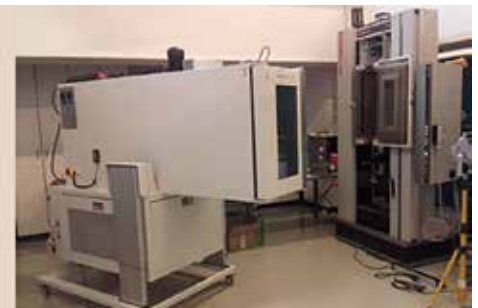
Fig. 2 right: Test equipment for mechanical material characterisation under real operating conditions (mechanical loads, temperature and humidity ranges)
