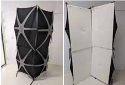
Fig. 1 above: Test arrangement for ballistic tests on component modules in the shooting channel Fig. 2 left: Demonstrator modules as an assembled protective structure after shooting with 9 mm calibre (645 m/s and 1662 J)
