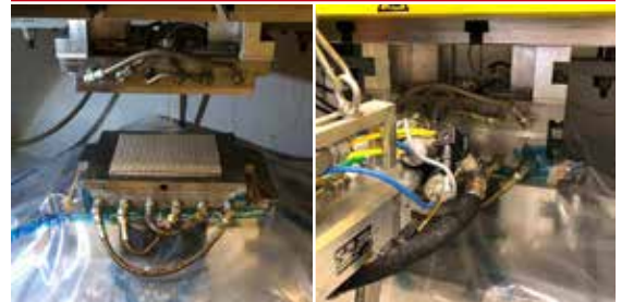
Above: Processing of natural fiber reinforced composite using 100% bio-based resin by vacuum assisted resin infusion Below: Processing of recycled sandwich composites using RTM process
