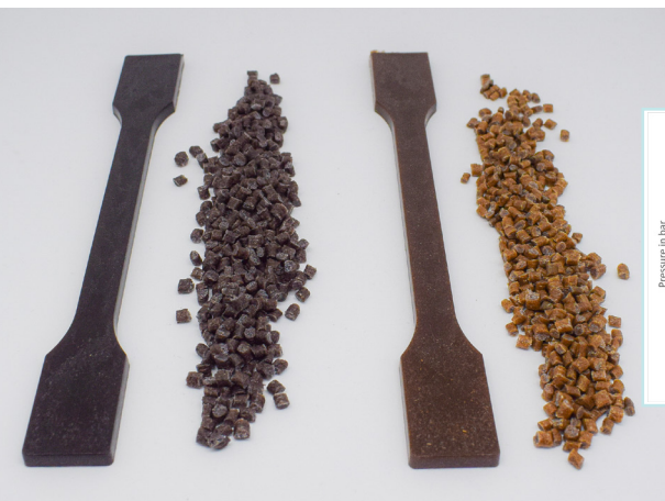
left: Granulate and test specimens made from the bark of fir (left) and elephant grass (right) / right: pressure at the screw tip of the different fillers
