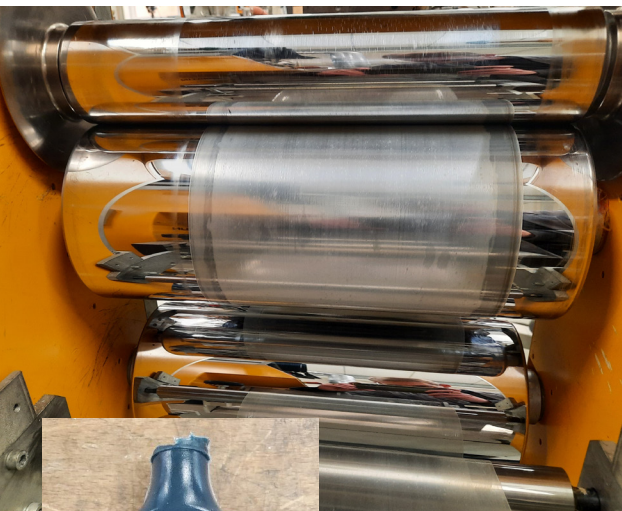
above: Film extrusion with recycled material left: Bottle made from recycled material
