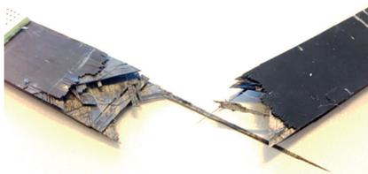
Fatigue failure of a quasi-isotropic laminate
