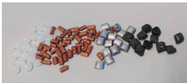
Polymeric thermal energy storage material containing different fillers
